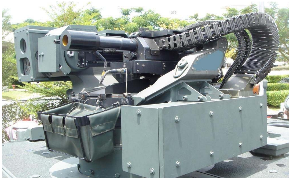
EOS R-600 Dual Weapon System with 40 mm AGL and 7.62mm GPMG
